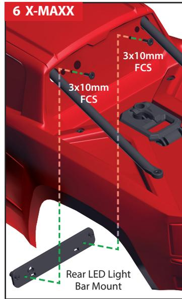
Install the rear LED light bar mount on the truck body using the two included 3x10mm flat-head screws.
